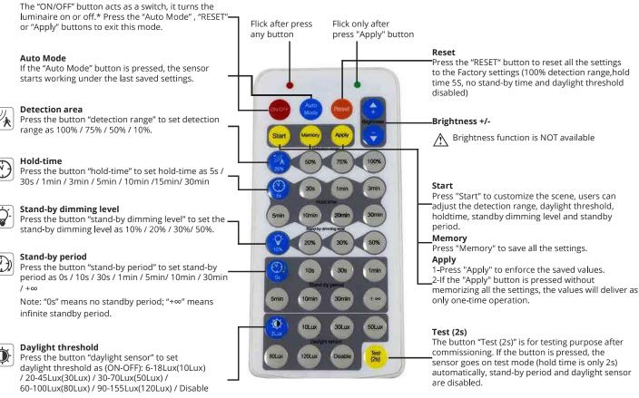
Note: Disable means light will be turned on once the sensor detects movement, regardless of the ambient daylight lux levels.
